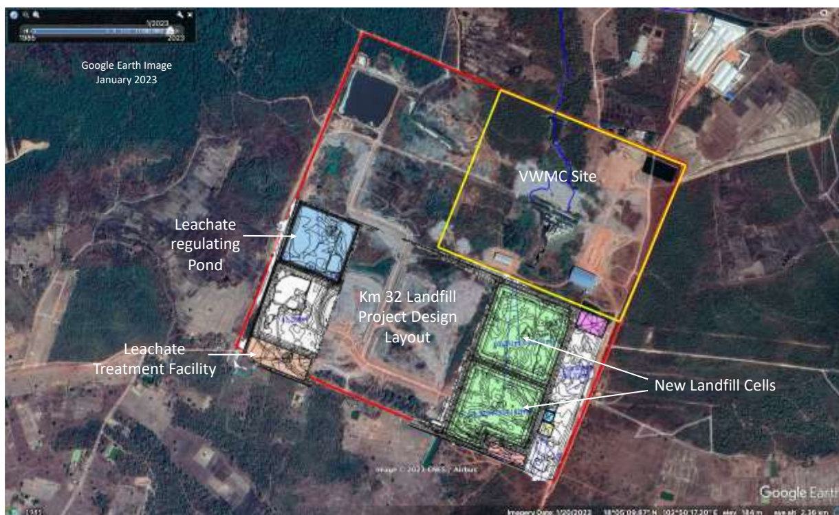
FIGURE 4-7 THE CONCEPTUAL LANDFILL DESIGN SUPERIMPOSED ON A GOOGLE EARTH IMAGE, 2023
