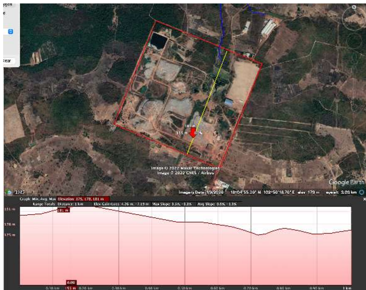
FIGURE 6-10 TERRAIN PROFILE OF THE KM 32 LANDFILL ACROSS THE VCOMS AND KHOUANMOUANG COMPANY SITES
