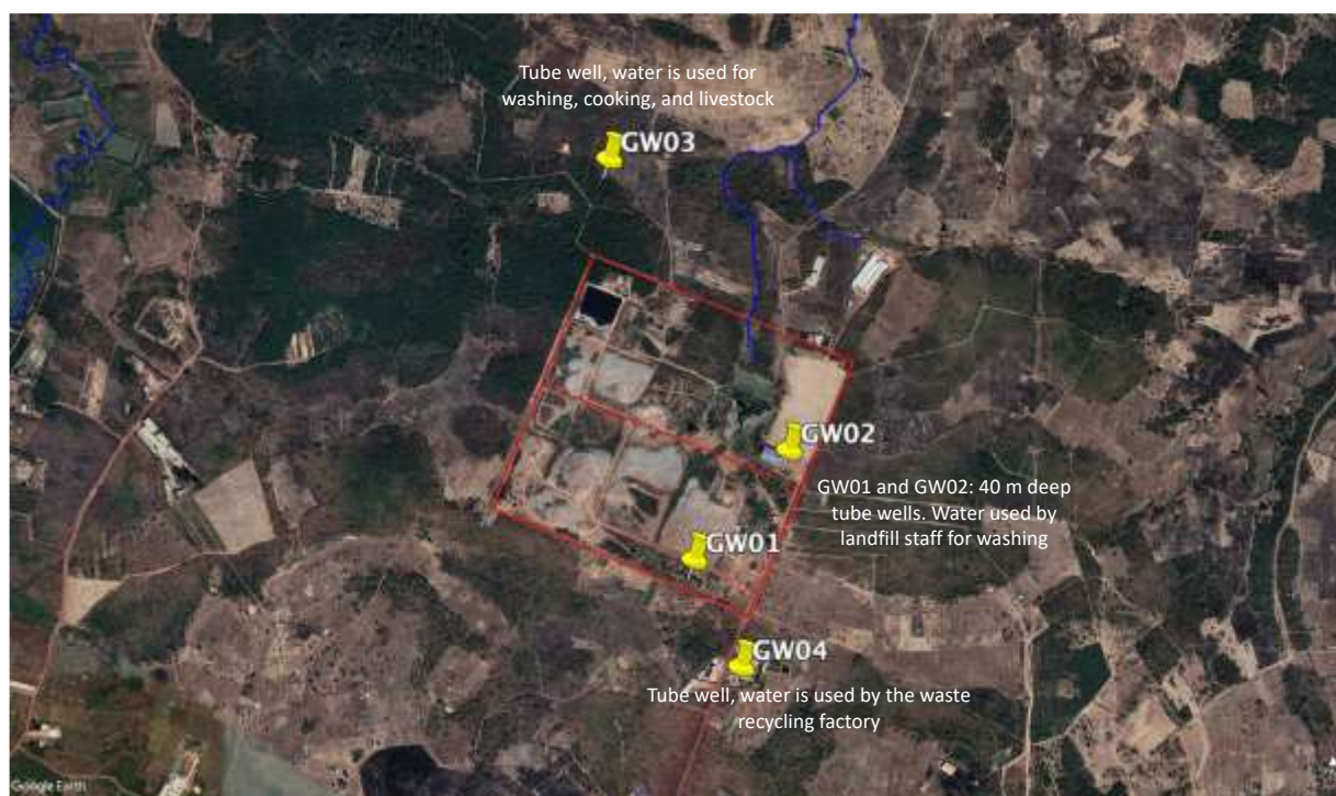
FIGURE 6-20 GROUNDWATER WELLS MONITORED UNDER THE PRE-FEASIBILITY STUDY
