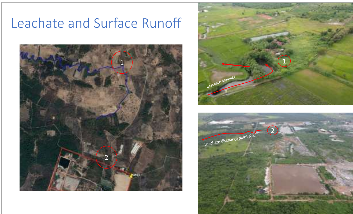
FIGURE 6-17 LEACHATE DRAINAGE FROM THE NORTHERN PART OF THE KM 32 LANDFILL
